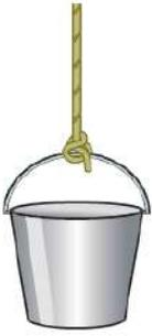
$$\begin{aligned} \Sigma F = 0 & \quad \left| \quad F_T = F_g \right. \\ & \quad \quad \quad = m \times g \\ F_T - F_g = 0 & \quad \left| \quad \quad \quad = 12 \times 10 = 120 \text{ N} \right. \end{aligned}$$
